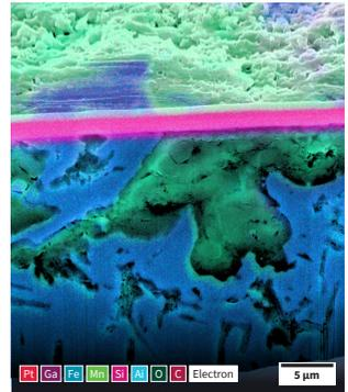
Overlay images of EDX (elemental identification) results on top of SEM image
